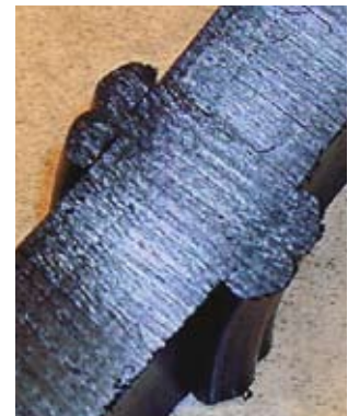
Weld beads on a PE pipe; cross section through a joint
